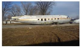
In June 2017, several Ghost Squadron volunteers began work by power-washing the years of built-up dirt from the outer surface of the fuselage in preparation for painting the fuselage. The plan was not to paint the entire fuselage, but only areas where any markings of importance would be placed. This included the areas at the rear of the fuselage on both
